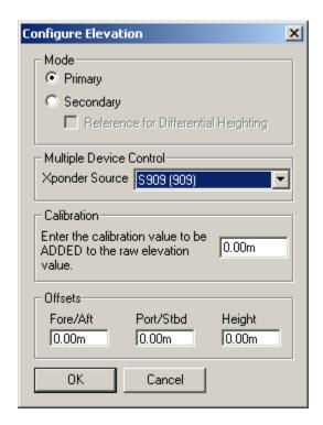
If in the above, the XPONDER has been configured for *Use in differential depth mode...* this data item is set to *Secondary* and the *Reference for Differential Heighting* box is checked. The transponder selected as the *Tracking Transponder* in the XPONDER configuration is then selected from the drop down list in the *Multiple Device Control* panel.
