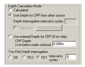
When this option is selected, the *Tow Fish Depth Interrogation* section of the panel becomes enabled. The configuration for the *other source* is done here.
