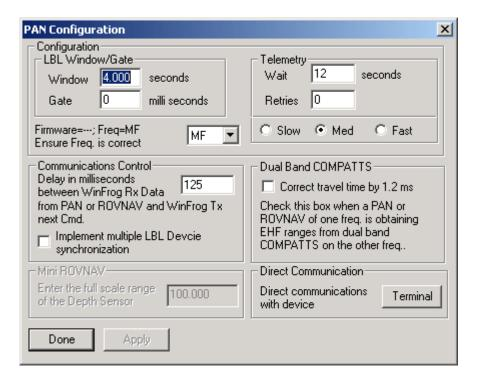
The Slow, Medium and Fast radio buttons set the telemetry baud rate through the water. See Pan manual for details on the BN and BF and BS commands. When the PAN device is first selected for use it automatically send the commands mentioned above to initialize the PAN
