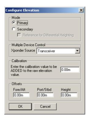
When being used with an XPONDER data item configured for *Use Depth of CRP from other Source* or *Interrogate Depth/Attitude Only*, this data item is set to *Primary* and the transponder selected as the *Tracking Transponder* in the XPONDER configuration is selected from the drop down list in the *Multiple Device Control* panel.
